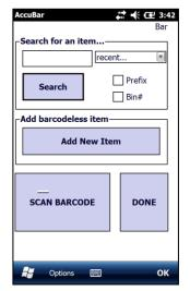
Scanning barcodes takes practice and you may need to move the handheld closer to or further from the actual barcode, or up and down until it reads it; generally a distance of about 8" is best. You will only be scanning items that have barcodes for now. DO NOT scan barcodes of case products at this time.
